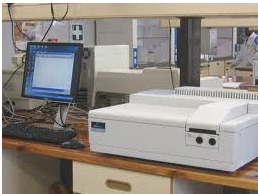
Fig. 1. The spectrophotometer UV/VIS Perkin Elmer Lambda 25
