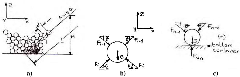
**Fig.2.** The arrangement of apples in rows corresponding spherical model rhombic arrangement (a); scheme of forces acting on an apple in the row (rows are numbered starting on the surface of the containers) (b), scheme of forces acting on an apple on the last row (c)
