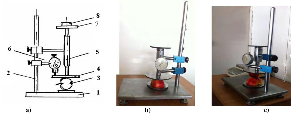
**Fig. 1.** Creep apparatus: 1 - device frame; 2 - support; 3 - apple; 4 - compression rigid surface; 5 - guide; 6 - dial gauge; 7 - plane; 8 - constant load.
