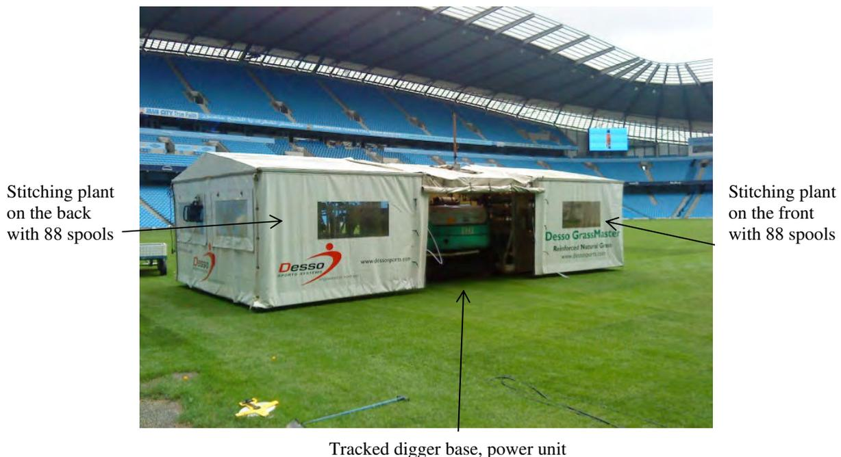
The computerised system works in a cycle operated by hydraulics and pneumatics. In each cycle a thread of fibres is fed through, cut to the correct length and injected into the pitch, then the machine moves forward and the process continues.
