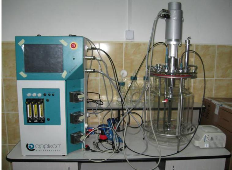
**Fig. 1.** Laboratory-scale bioreactor for submerged fermentation
