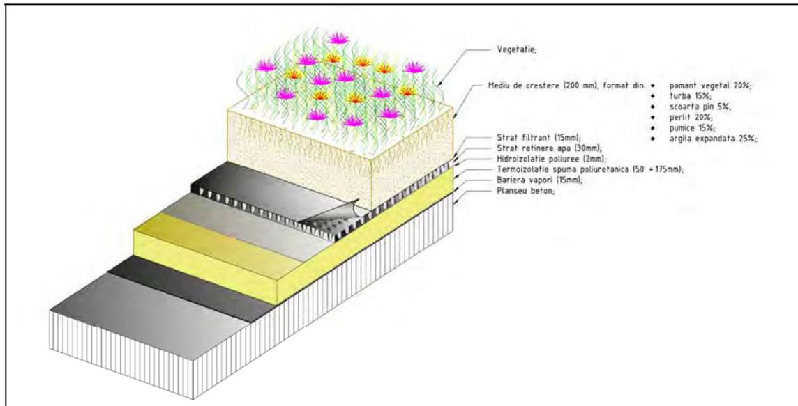
Fig. 2. General structure to implement the layers of a green roof
