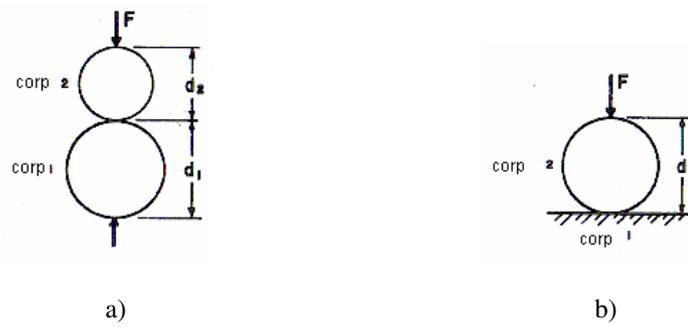
**Fig.1.** Elastic contact for two convex bodies, sphere on sphere (a), sphere on flat plate (b)
