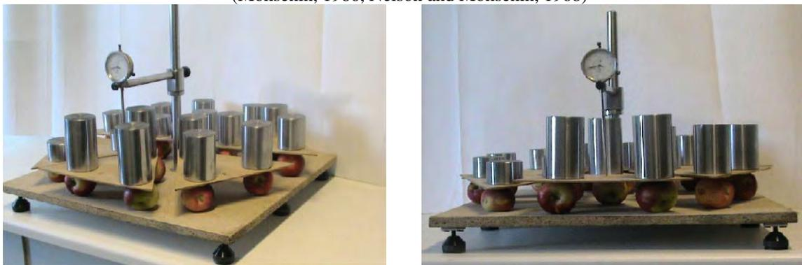
**Fig. 3.** Dead load testing apparatus
