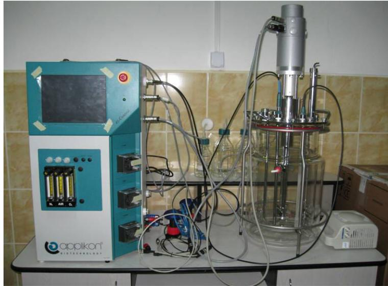
**Fig. 1.** Laboratory-scale bioreactor for submerged fermentation
