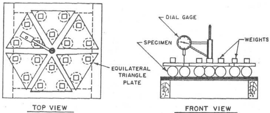
**Fig. 2.** Apparatus for measuring distortion of fruits under dead load (Mohsenin, 1986, Nelson and Mohsenin, 1968)
