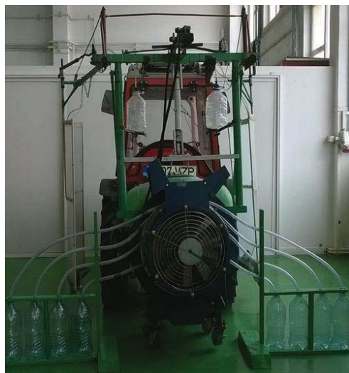
Figure 2. Collection of each nozzle spray solution on the two ramps spraying machine for pest and disease control in vineyards TARAL 200 PITON TURBO
