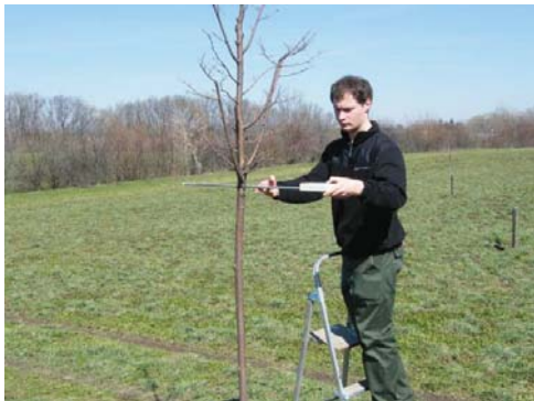
Figure 1. Measuring with AccuPAR LP-80 linear ceptometer (12.03.2014., Soroksár)
