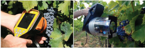
Figure 3. (A) Spectron. (B) Multiplex hand device sensors for grape quality proximal monitoring, which allows quality maps to be realized (Matese and Di Gennaro, 2015)
