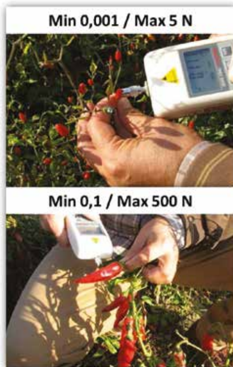
Figure 1. Measuring of FDF using push-pull digital gauge
