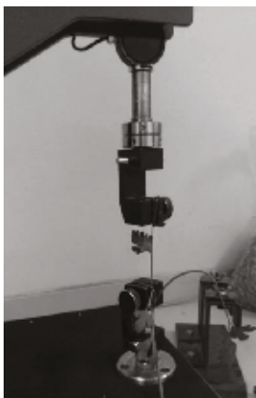
Figure 5. Measuring the picking force of parsley ( Petroselinum crispum ) leaf stalk
