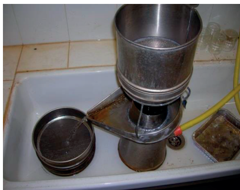
Figure 1. Apparatus of Fenwick for cysts extraction
