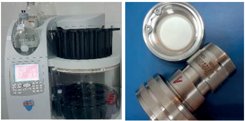
Figure 3. ASE 350 system and extraction cell
