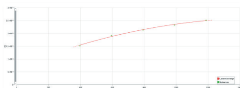
Figure 8. Calibration curve for the trans -resveratrol standard (UV \lambda 320 nm, without derivatization). Polynomial regression, equation: y = -7.998 \times 10^{-15}x^2 + 2.472 \times 10^{-8}x + 6.9 \times 10^{-3} , coefficient of variation (CV): 1.21%, correlation coefficient (R): 0.997286
