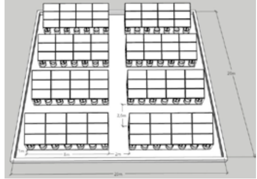
Figure 8. Rooftop with M12 modules
