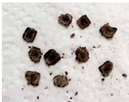
Figure 4. Granules after compression test
