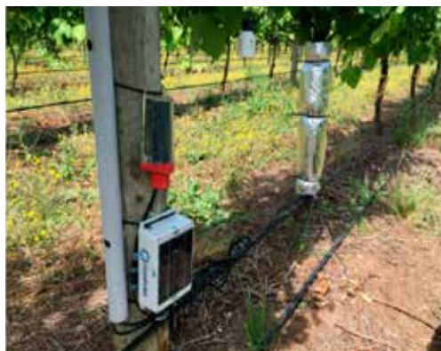
Figure 4. Close up view of an individual microtensiometer. MT data of trunk water potential ( \Psi_{\text{trunk}} ) (Vinay Pagay, 2021)
