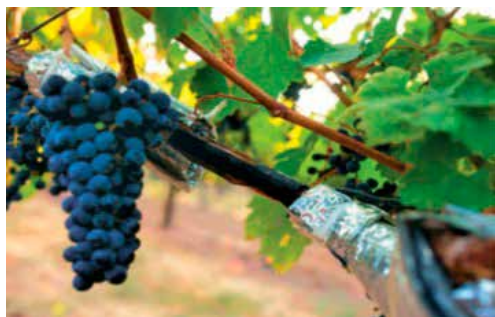
Figure 3. Close-up on a sap flow sensor placed on a lateral vine branch. The heating tab surrounds the entire section of the branch. Temperature sensors measure the amount of heat displaced by the sap (after Ginestar et al., 1998; Scholasch, 2018)
