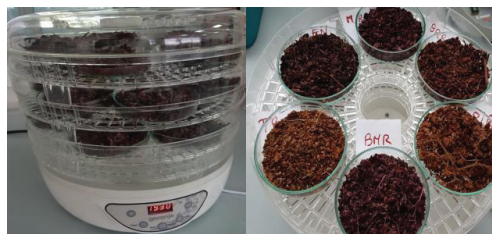
Figure 1. Grape marc dehydration in Gorenje FDK24DW Food Dehydrator
