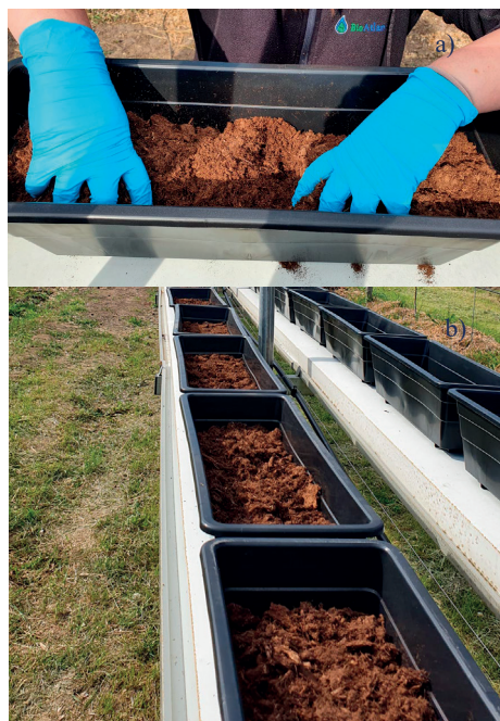
Figure 2. Filling pots with peat: a) crushing the peat; b) pots with crushed peat
