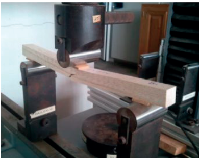
Figure 5. Determining of fiber resistance to bending
