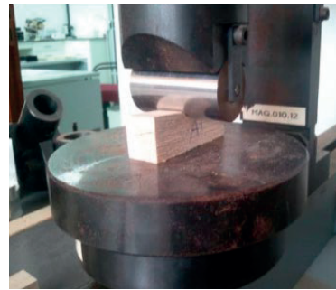
Figure 3. Determining the physical hardness of the fiber
