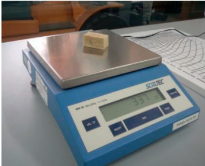
Figure 2. Determining of specific humidity and weight
