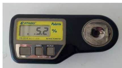
Figure 2. Determination of soluble dry matter, using the Atago refractometer (own source)
