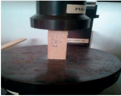
Figure 4. Determining of fiber resistance to linear compression
