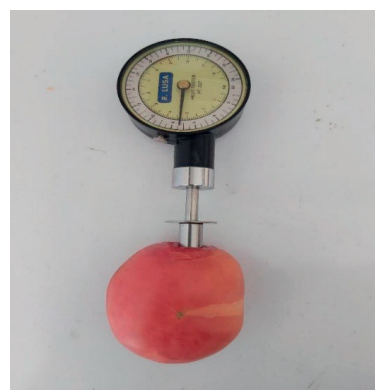
Fig. 3. Determination of fruit firmness, using the hand-held Effegi penetrometer (own source)
