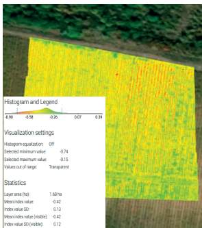
Figure 9. Determination of the Normalized Difference Water Index (NDWI)
