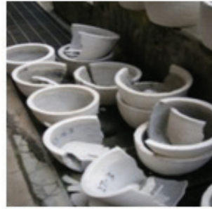
Figure 8. Test of Strength Vetiver Waste Pot
