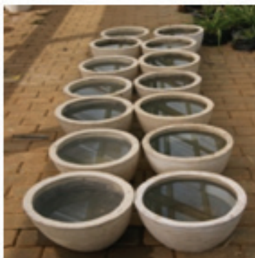
Figure 7. The Seepage Test of Waste Vetiver Pot
