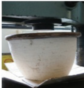
Figure 8. Test of Strength Vetiver Waste Pot
