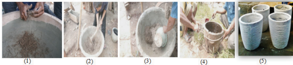
Figure 2. Manufacture of vetiver waste process (1) Vetiver waste is cut in to small pieces (2) Vetiver waste is mixed with cement and sand (3) Stir it so that the dough distribute evenly (5) The printing dan (5) And that is teh eco-friendly vetiver waste pot.
