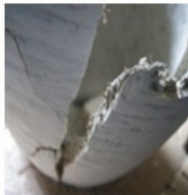
Figure 9. The Pot Condition After Pressing Test
